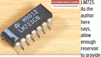
the base current. Often we see an additional supply for the output series pass, the regulator circuitry and as we shall see, the 'lift' voltage to put the LM723 above rail if the output voltage is needed to go down to zero volts. (it's easy with a Voltage Reference voltage divider to get the output down to +2Volts, but down zero is a whole different situation. There is a video to watch. Really well made video
