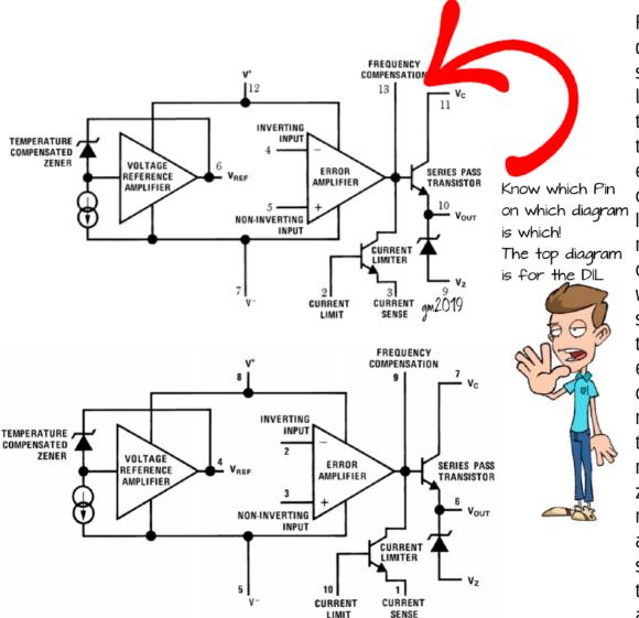
From this lower diagram we can see that the LM723 contains the op amp, pass transistor, reference voltage circuit and current limit transistor needed for the circuits that we've looked at so far in this section. The reference voltage circuit is a little more sophisticated than just a resistor and zener diode connected in series and so it is simply shown as a functional block with a 7.15V output.
