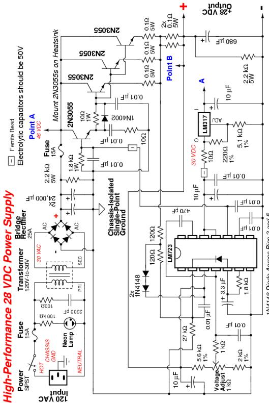
ing the circuit to show what the LM723 is doing. When looking at this circuit it's awkward to know what is happening. For example: Look at the LM317 regulator. Is the output going to point A? No it is not! Point A is the input to the LM317 and it is being used like the circuits we already saw, to supply the LM723 with a steady regulated voltage supply of  $30V_{dC}$ . Why are so many 2N3055 transistors used? You can read ്യ more about this supply
