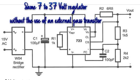
current limit and R3 with R4 set the output voltage.
